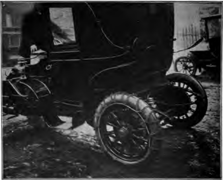
FIG. 46.—Anti-skidding device on the rear wheel of a Mercedes limousine. A network of steel chain offers sufficient resistance to prevent side-slip and skidding on a snowy street
